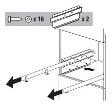
Position the rails on the sides of the cabinet as shown in the figure. Fix with the screws supplied, then extract them completely. If the coffee maker is installed over a warmer drawer, use the top surface of this as a reference to position the rails.
