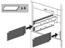
If necessary, correct alignment of the appliance by positioning the spacers supplied under or at the sides of the support.
