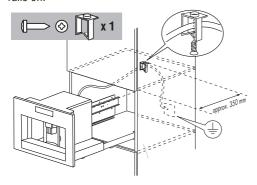
Fix the power cable with the clip.
